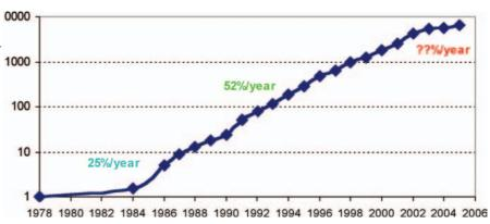
Growth in processor performance since 1978 relative to the VAX 11/780 as measured by the **SPECint benchmarks** (from SPECint89 to SPECint2000). Prior to the mid-1980s, processor performance growth was largely technology driven, and averaged about 25% per year. The increase in growth from 1986 to 2002 to about 52% was due to more advanced architectural and organizational ideas exploiting Moore's Law. It's less than 20% per year since 2002 [3].
